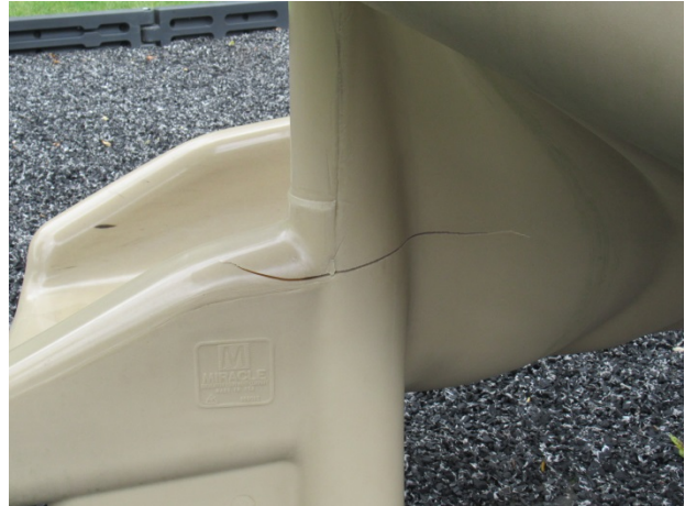
Crack at the slide
